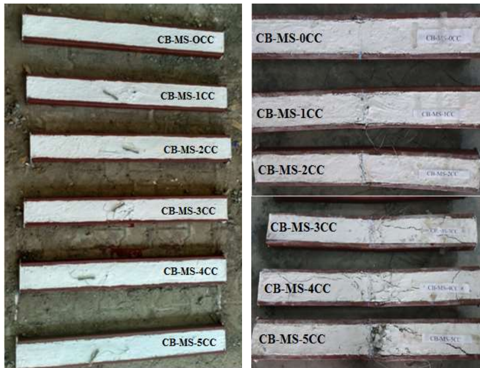
Fig. 5. Cold-formed steel-composite beams before and after testing
