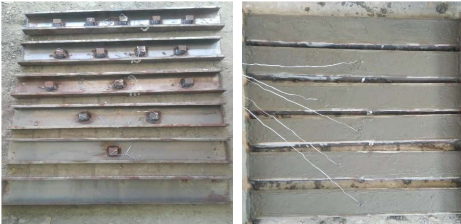
Fig. 3. Samples with a strain gauge on the channel shear connectors
