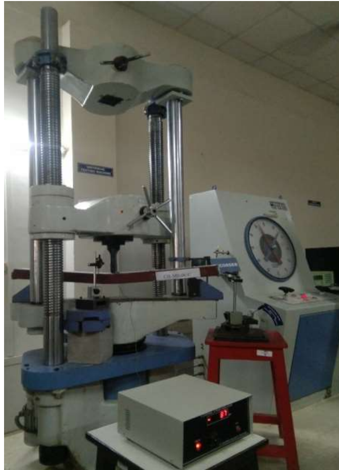
Fig. 4. Cold-formed steel-composite beam under testing using UTM
